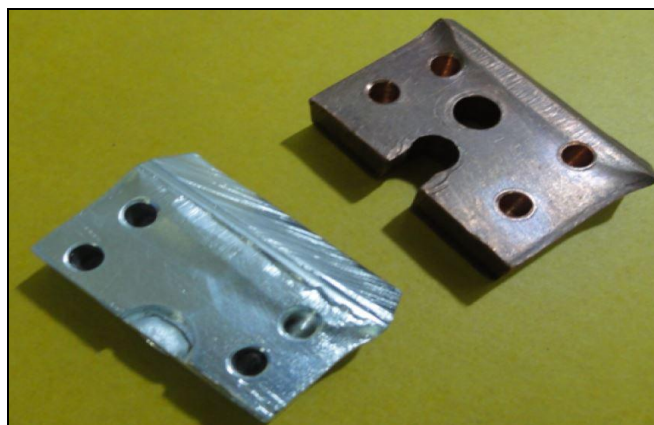
Fig. 10. Tin coated and without coated sample
