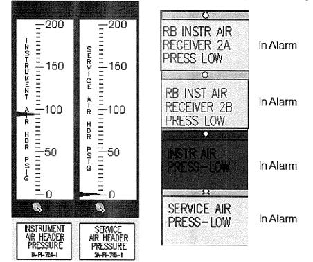
Which one of the following identifies the required operator action IAW 0AOP-20.0, Pneumatic (Air/Nitrogen) System Failures?
