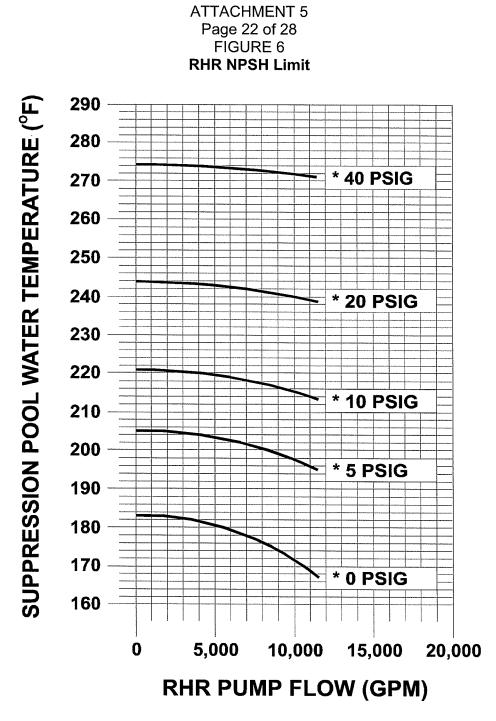
SUBTRACT 0.5 PSIG FROM INDICATED SUPPRESSION CHAMBER PRESSURE FOR EACH FOOT OF WATER LEVEL BELOW A SUPPRESSION POOL WATER LEVEL OF -31 INCHES (-2.6 FEET).
