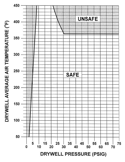
DRYWELL AVERAGE AIR TEMPERATURE MAY BE DETERMINED USING ATTACHMENT 4.
