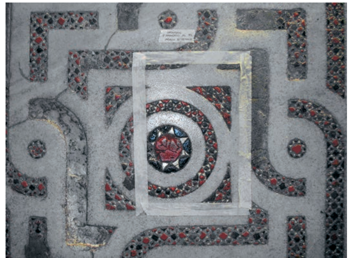
FIGURE 5 Result of cleaning test with a poultice of a 7 percent ammonium bicarbonate solution applied for fifteen minutes.
