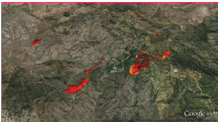
Figure 2 —FireMapper thermal image of the Esperanza Fire, showing ground surface temperatures as viewed from above on October 26, 2006, between 14:07 and 14:17 PDT.
