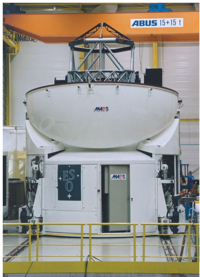
Figure 1: The first Auxiliary Telescope for the VLTI during final testing at AMOS in Liège (Belgium).
