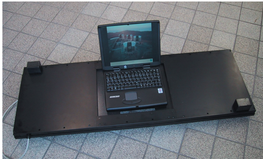
Figure 4: The OmegaCAM exposure shutter. The aperture size is 370 \times 292 mm, the shortest possible exposure time is smaller than 1 msec, the deviations of the effective exposure time from pixel to pixel (homogeneity) are smaller than \pm 0.2\% for a 100-msec exposure, the exposure time accuracy is about 0.3 msec. (The laptop computer gives an idea of the scale.)
