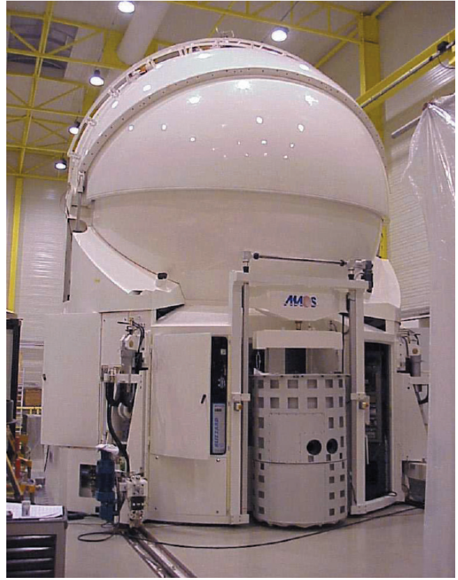
Figure 6: The Transporter in its relocation configuration. The cylinder in the foreground houses the Relay Optics and the coudé sensors (CCD and STRAP). The light beam exits the telescope by one of the two black openings. During relocation, the cylinder is lowered underground inside the station pit before the telescope is placed on top.
