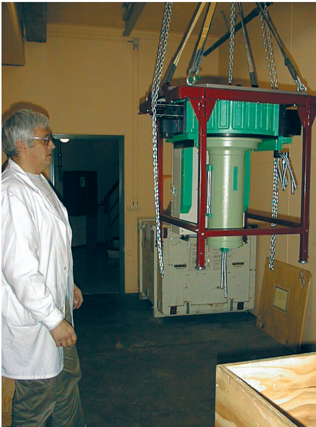
Figure 1: The finished HARPS Cassegrain Fibre Adapter ready to be shipped from La Silla to Geneva for system tests.
