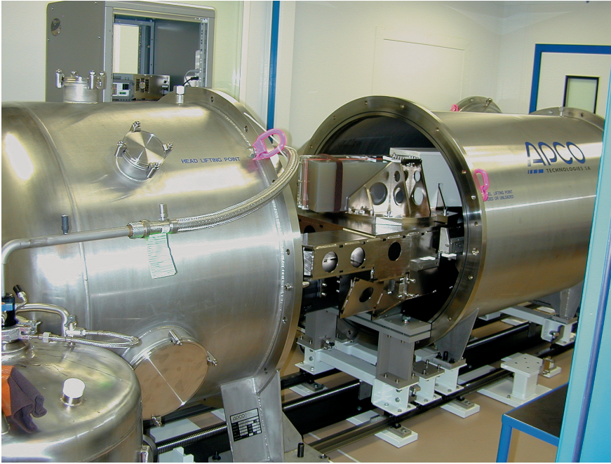
Figure 3: The open HARPS vacuum vessel. The back side of the echelle grating is visible on top of the optical bench as well as the rail system used for moving the large parts of the vessel.
