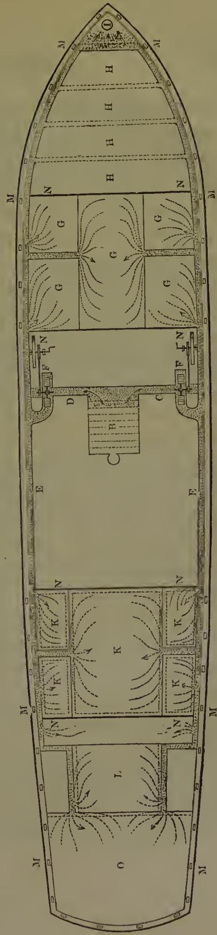
arrived in the Niger. The letter **F** represents the fanner or ventilating machine, receiving the vitiated air from the various compartments of the ship, and discharging it at **s**.
