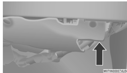
Interior Fuse Panel Location
