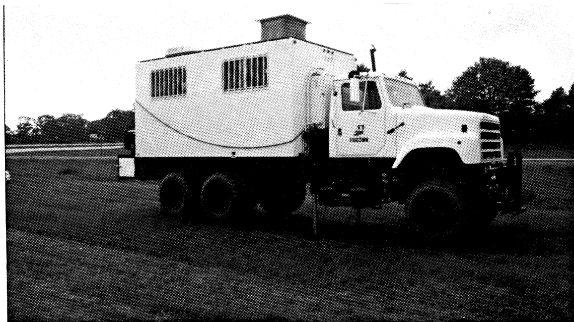
Figure 4.10. Van den Berg Type Cone Truck at Louisiana Transportaton Research Center.
