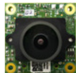
e-CAM24_CUNX - Color Global shutter Camera for,NVIDIA® Jetson Xavier™ NX / TX2 NX / Nano
