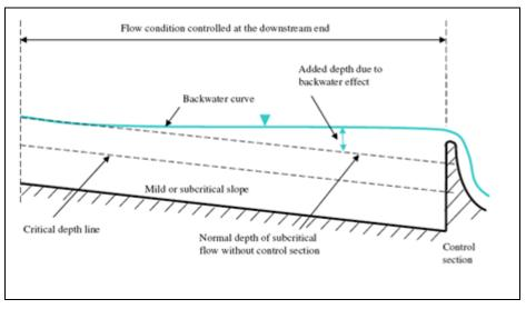
Figure 6.6 Schematic diagram of the back water curve
