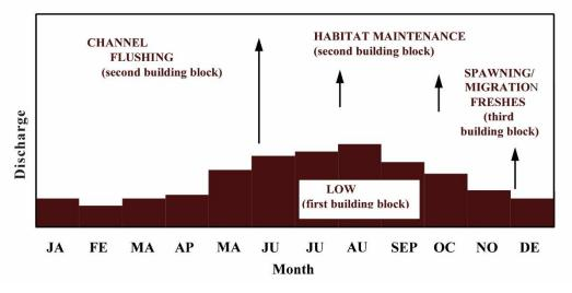
Figure 11.1. Example of flow regime built up using building blocks
