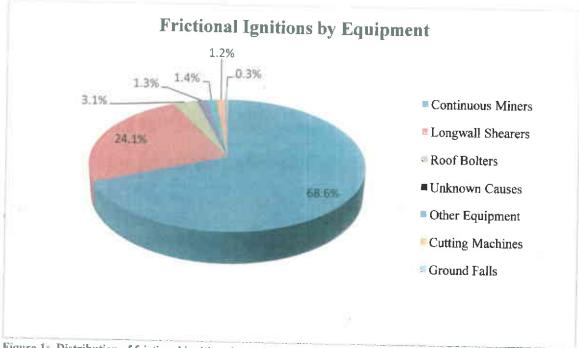
Figure 1: Distribution of frictional ignitions by equipment type, 1983-2005. Data from Krog and Schatzel, 2006.
