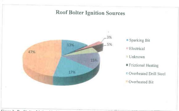
Figure 3: Roof bolter frictional ignitions 1981-1998. Data from Urosek and Francart, 1999.
